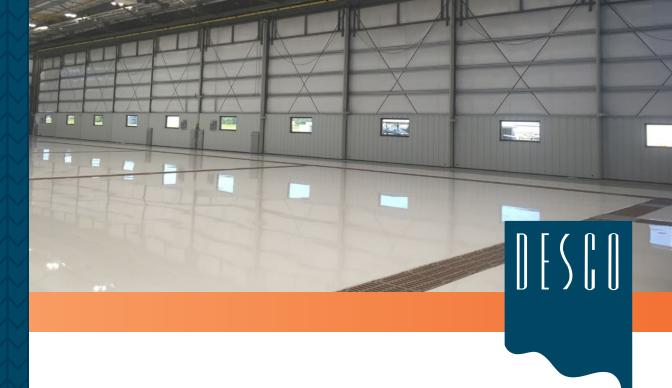
**DESCO INDUSTRIAL SERIES CA** is a High Wear fluid applied thermosetting flooring coating system that can be installed over any sound concrete surface at an economical price. This product possesses exceptional resistance to wear, abrasion and to most acids, alkalis and solvents.
