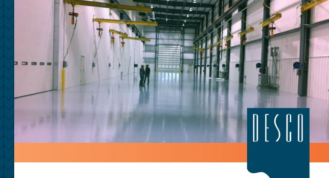
**DESCO INDUSTRIAL TG** is a trowel grade thermos setting flooring material that is a solid color resin. It can be applied over rough to smooth concrete surfaces either by hand trowel or power trowel. This system is offered with the leading stain resistant finish coats if needed. It is normally applied at 1/8" to 1/4" thickness.
